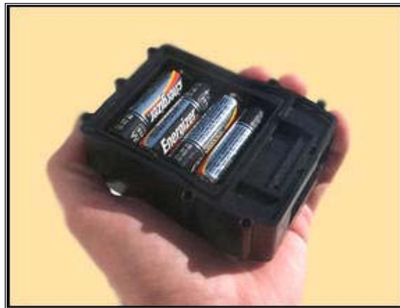
Figure 2. LandAirSea 3100-INT Passive GPS Unit.
