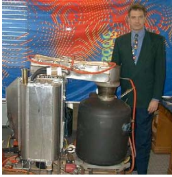
Figure 6: Zeo-Tech's prototype Zeolite Heat Pump
