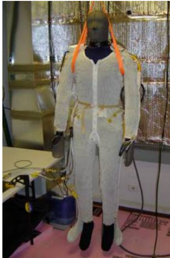
Figure 36. ADAM in a NASA Liquid Cooling Garment
