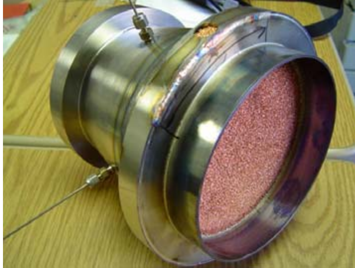
Figure 26. Copper foam heat exchanger for a thermoacoustic system
