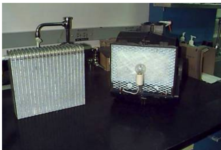
Figure 29. A prototype photocatalytic air-cleaning system
