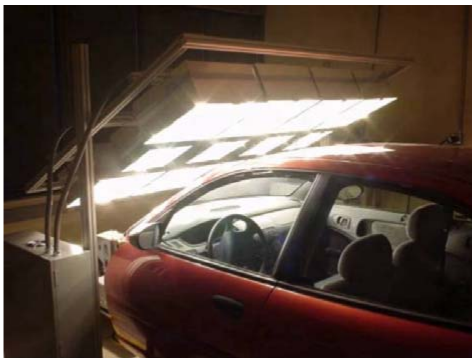
Figure 18. Vehicle Climate Control Laboratory with solar lamps
