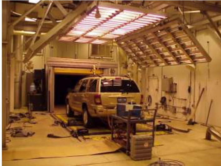
Figure 44. Chrysler Environmental Test Cell with IR lamps
