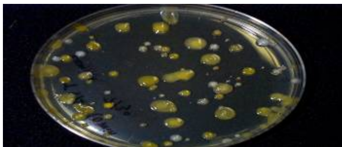
Figure 27. Bacterial growth from a 10-minute A/C vent outflow
