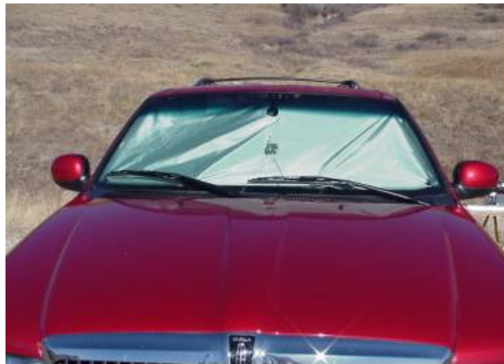
Figure 17. Solar-reflective shades in a Lincoln Navigator
