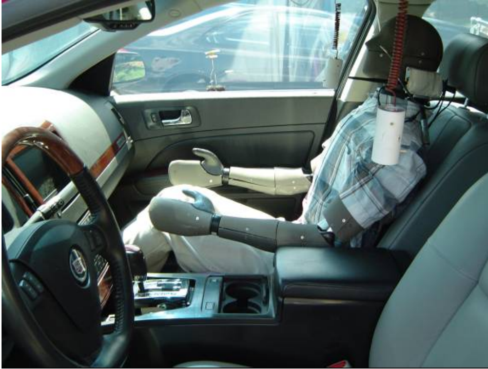
Figure 19. ADAM testing a W.E.T. ventilated seat
