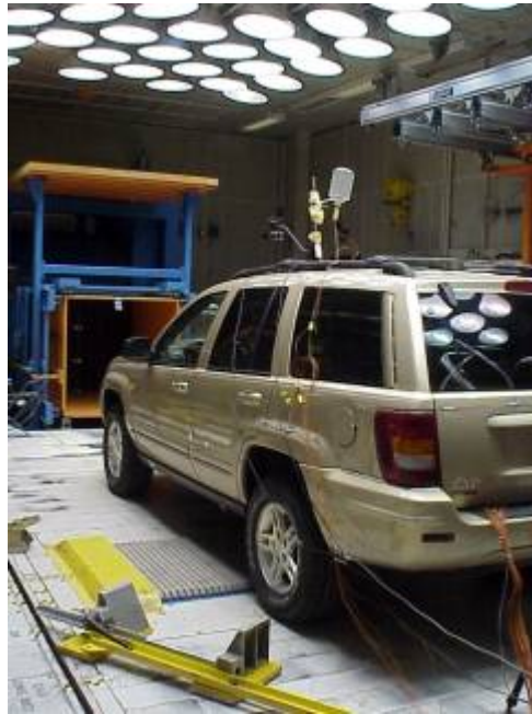
Figure 43. Chrysler Emissions Test Cell with metal halide lamps
