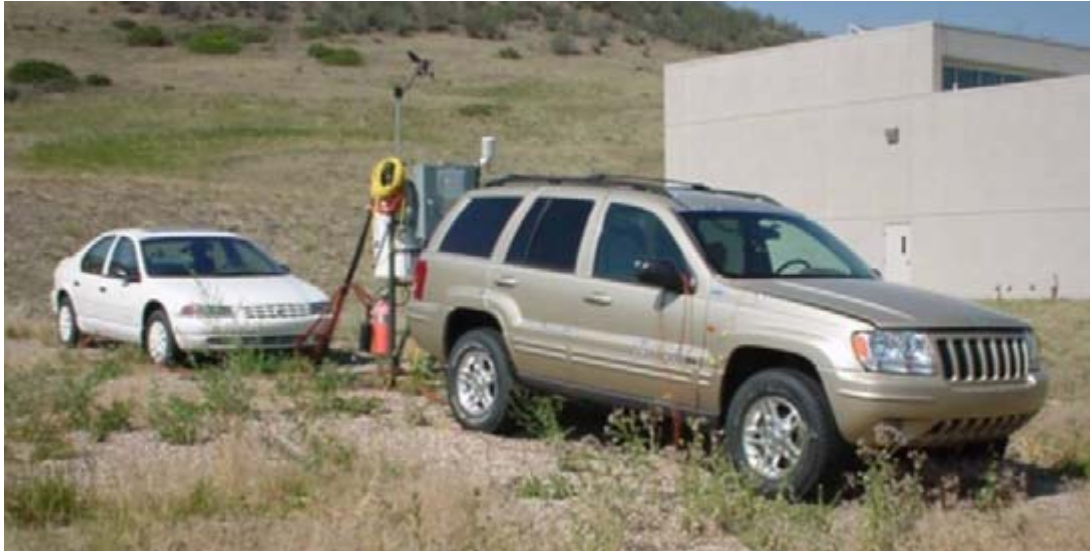
Figure 13. Jeep Grand Cherokee ventilation test setup
