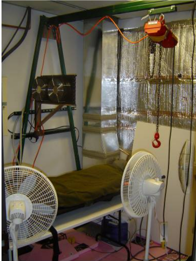
Figure 40. NREL's Manikin Environmental Chamber
