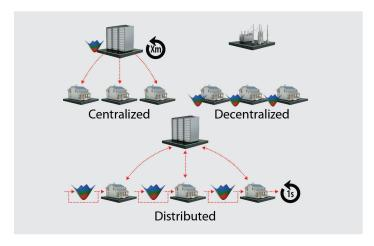
The real-time optimization architecture offers distributed decision-making capabilities while systematically coordinating the operations of DERs to increase reliability. This is in contrast with centralized and decentralized control systems. Illustration by Josh Bauer, NREL.
