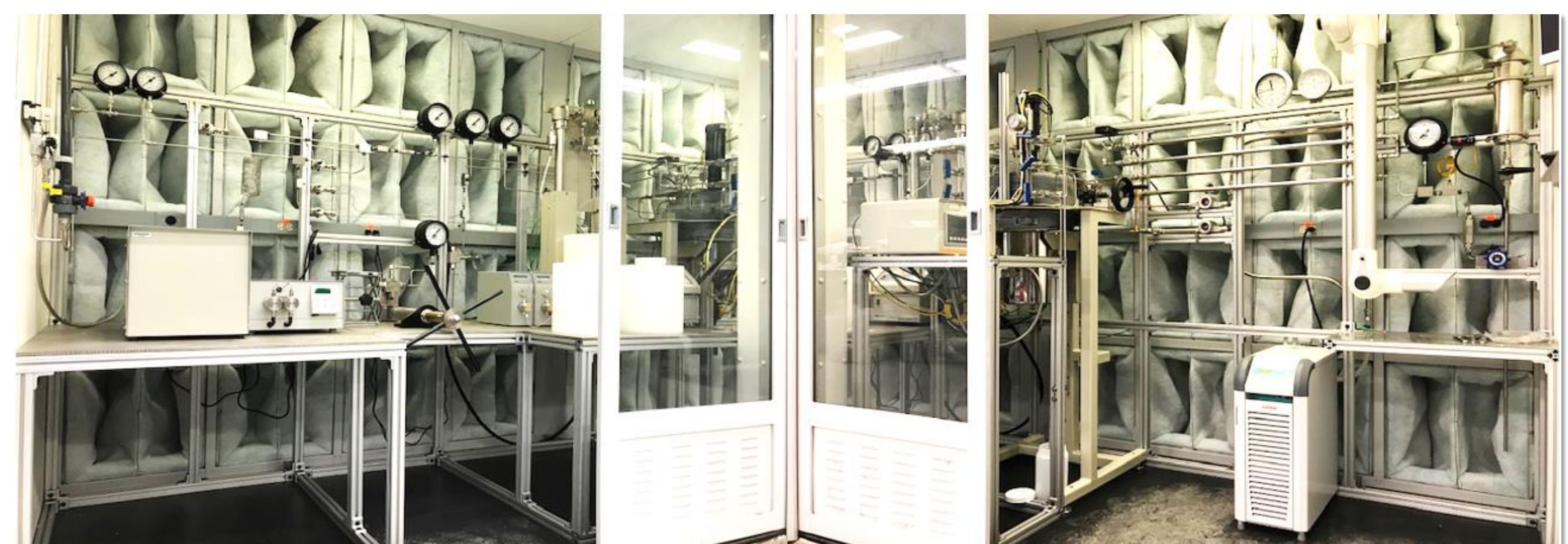
Fig. 5. Multi-purpose batch-type supercritical fluids processing system at ANL MERF
